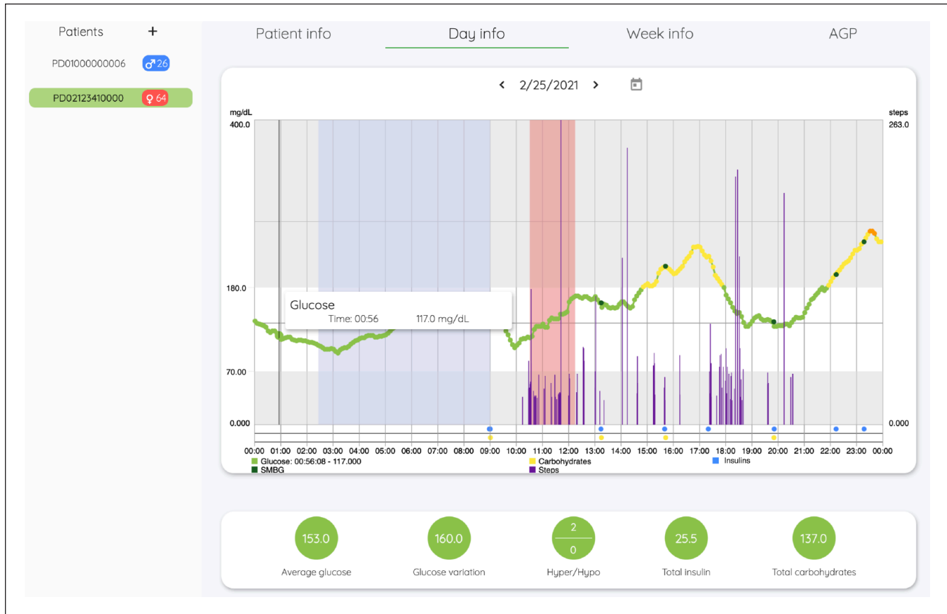
Figure 3. Main page of the IMPACT web interface. On the left panel, each patient can be selected, and new patients can be enrolled in the trial. On the central panel, 4 subpanels allow to access to different information, that is, patient demographics, data collected in a specific day, data collected in specific week, and AGP report. On the bottom panel, statistics about the selected portion of data are provided.
